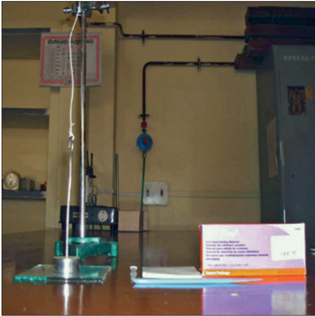
Fig 1 Load placement on glass plate containing sealer.
