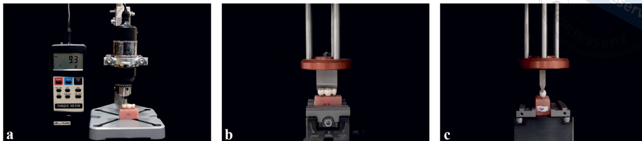
Fig 4a to c Cyclic loading test. An electronic torque meter was used to measure loosening torque values of restoration screws (a); frontal view of cyclic loading on the central fossa of the three-unit ISFDP (b); lateral view of cyclic loading on the central fossa of the three-unit ISFDP (c).
