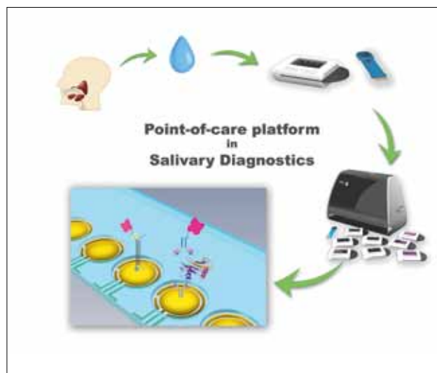
Fig 1 Illustration of the point-of-care platform for salivary diagnostics. The process requires that the saliva sample is put directly on the sensor cartridge; the on-site multiplexing detection of different types of biomarker is then carried out on the same chip.
